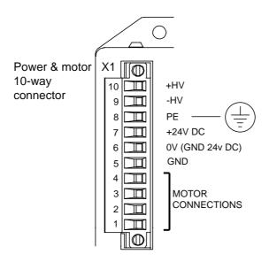
Figure 3-1. X1 Power Connections
